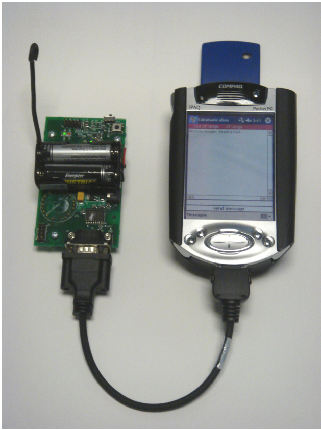
Figure 13: Mobile node with RFID reader
