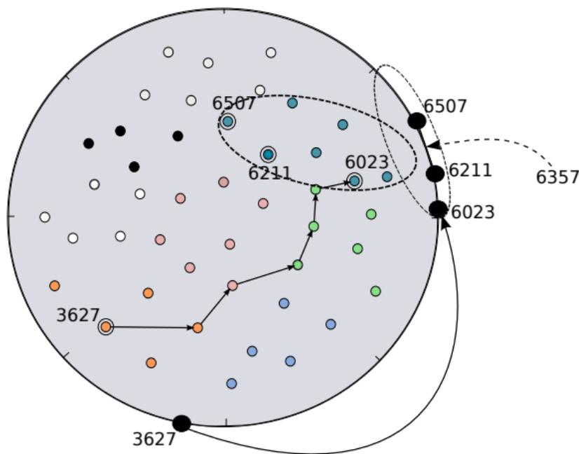
**Figure:** MADPastry Routing Example from 3627 to 6357 with Broadcast. After [6].
