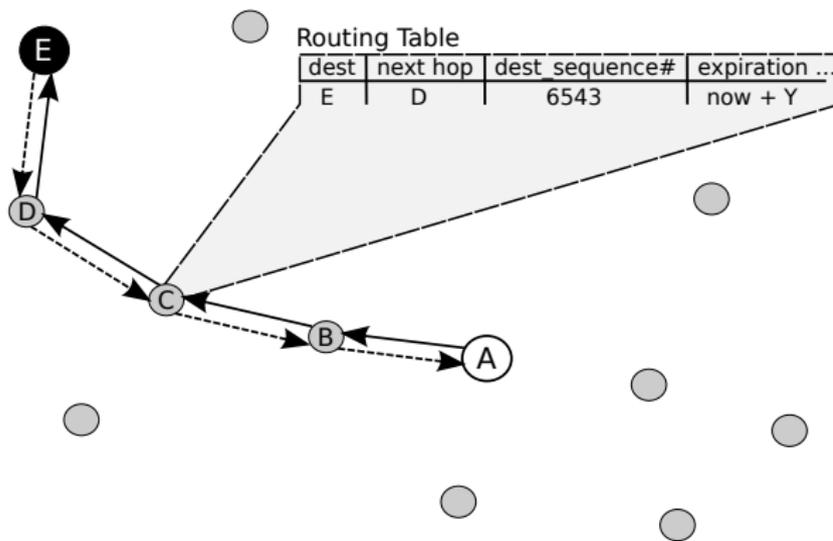
Figure: Forward Path Setup from A to E. After [2].
