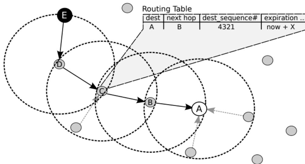
Figure: Reverse Path Setup from E to A. After [2].
