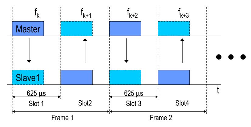
Complete packet transmission occurs during a Slot
