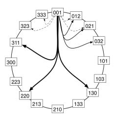
Figure 5: Graphical representation of a Pastry routing table from [20] where b = 2 and |L| = 4. Bold arrows represent entries from the routing table R, dashed arrows the leaf set entries in L.
