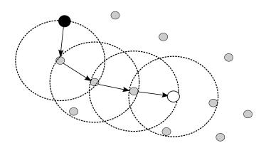
Figure 7: A RREQ is sent by the white node to discover a route to the black node. The route entries generated for the *reverse-path* are represented by the arrows.
