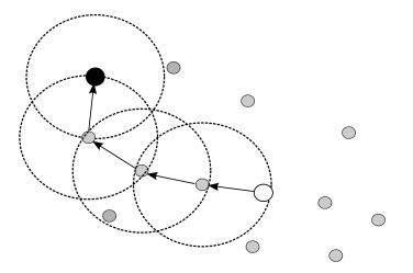
Figure 8: A RREQ arrived at the black node and it responds with a RREP along the route to the white node. The routes entries generated for the *forward-path* are represented by the arrows.
