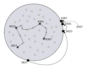
Figure 6: Routing with Pastry. Node 3627 is sending a message to 6257 which gets routed to the numerically closest node: 6367. The outer circle represents the overlay hops while inside the physical hops performed are shown.
