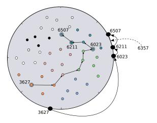
Figure 2: Message routing in MADPastry with K = 8 and B = 8 after [23]. Node 3627 is sending a message to 6357, which gets routed to the numerically closest node: 6507. The outer circle represents the overlay hops while inside the physical hops performed are shown.
